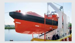
Because the safe working load and outreach of the davit is normally determined by the size of the rescue craft, be sure to check with your Sales Manager on the specific product application you are considering. All models provide easy access for periodic maintenance, service and repair, as well as clear labeling and detailed manuals.
