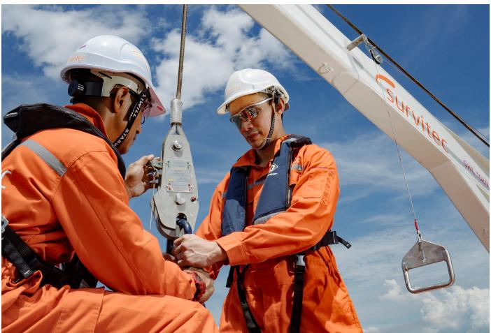
The Safelaunch SLA3.5 is an off-load fall-mounted automatic release hook for use with davit-launched liferafts and single-fall rescue boats.
