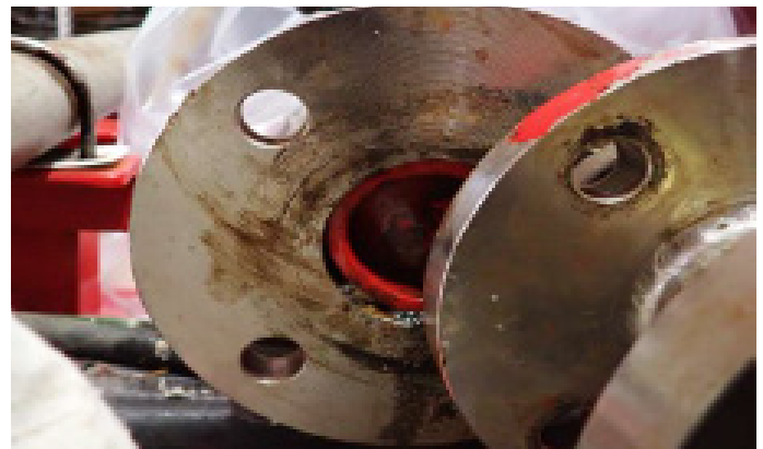
Figure 1. A protective cap (above, left) retrieved from inside a high expansion foam firefighting system (above, right), where it was restricting the flow of foam to the proportioner.
