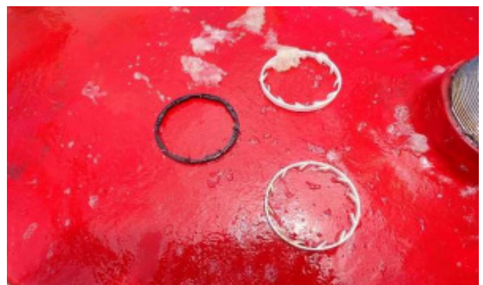
Figure 2. Internal inspection of the foam tank for a helideck foam system (above, left). In this particular instance, 60% of the foam was found to be in a gelatinous state after different types of foam had been mixed, rendering the system inoperable. The locking caps from the cans were found floating inside the tank (above, right).
